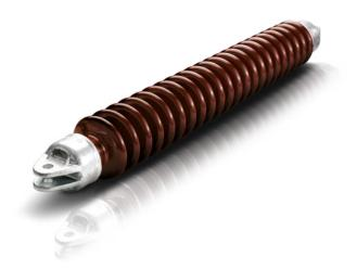
Longrod Insulators for transmission lines are produced in accordance with international standards and the respective customer specifications for high voltage transmission lines. In addition we design complete string sets from longrod insulators. To improve the performance under polluted conditions these insulators are also available with RTV silicone coating.
