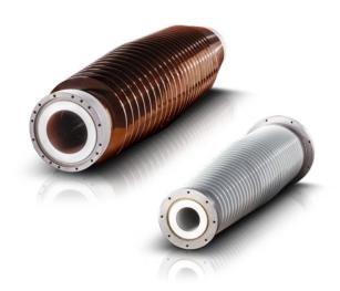
LAPP Insulators hollow core insulators are made of high strength C130 porcelain in accordance to IEC and ANSI standards. They are available in cylindrical, conical or round-bodied geometries up to a height of 2800 mm in a single piece.
